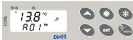
Starting from the normal condition (no alarms), when the instrument detects an alarm event, the left lower side shows the alarm code alternated with the probe value. The corresponding icon lighted.
