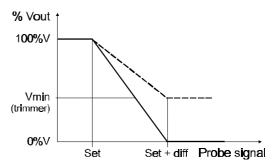
If the input signal is lower than the Set, the output signal is 230 Volt (fans are running at the maximum speed). When the signal increases and enters the range between the Set and Set+Diff the output signal follows the temperature variation. Above the Set+diff value the output signal is always 0 Volt (if no Vmin has been set).
