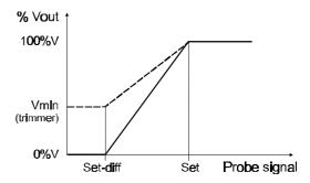
If the input signal is higher than the Set, the output signal is 230 Volt (fans are running at the maximum speed). When the signal decreases and enters the range between the Set and Set-Diff the output signal follows the temperature variation. Below the Set-diff value the output signal is always 0V (if no Vmin has been set).
