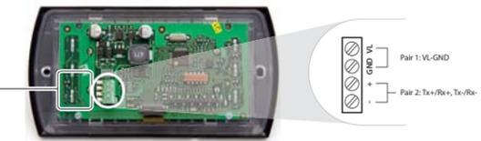
7. Finally, fix the pGD to the back piece folding the conductor only on the right side of the enclosure (front view)
